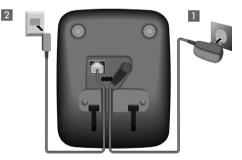
Only use the mains adapter and phone cord supplied. Pin connections on telephone cables can vary (pin connections → page 46). **First steps**
